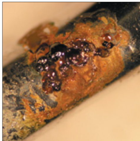
Figure 7: Newly purchased Desmarres corneal knife with corrosion
