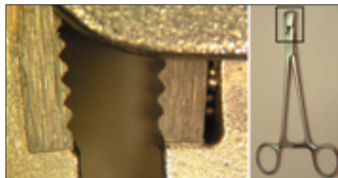
Figure 3: Wire holding forceps with poorly soldered insert
