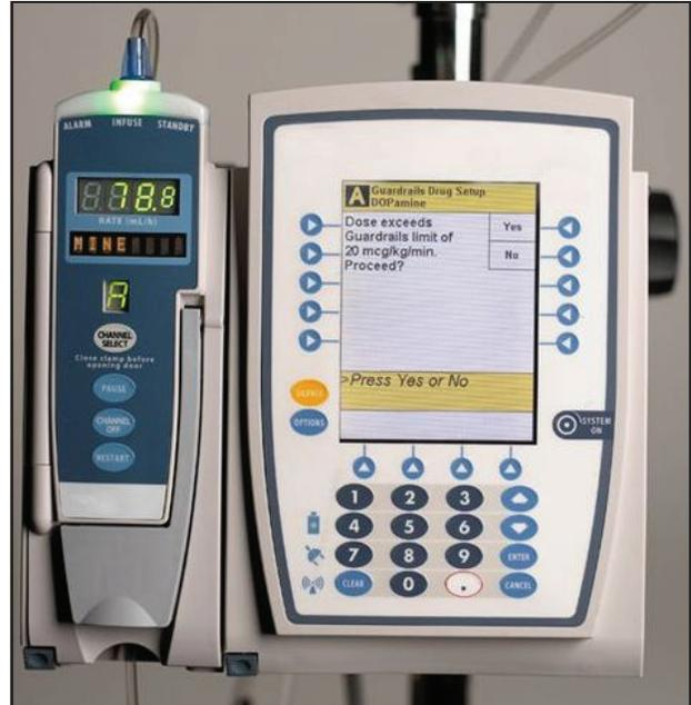
**Figure. Example of “Soft-Stop” Limit.** Image provided courtesy of ECRI Institute.
